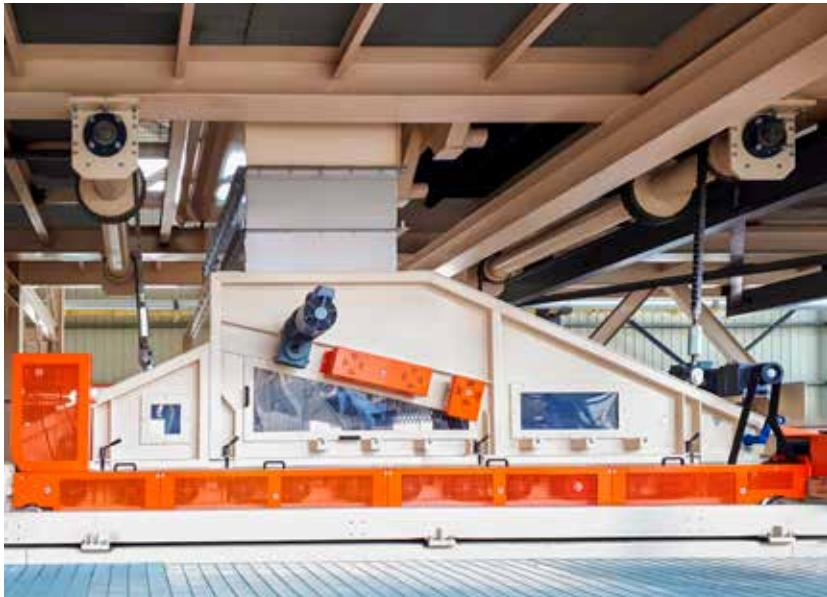
The OSB Dynaformer is used to form a uniform "mat" of oriented wood-based strands, resinated at a prior stage in the work process, which is then conveyed to the press.
