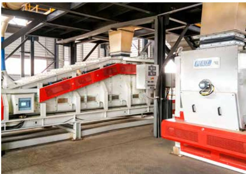
The machine is designed for the gravimetric dosing of material flows to feed, for example, drying or resin machines. The material is fed into a bunker of adequate capacity in which, thanks to a synchronized series of comb rollers and to the movement of a belt, it is fluidized until it forms a mattress of constant volume. Subsequently a weighing bridge with a high-precision load cell placed under the belt weighs the dosed material.
