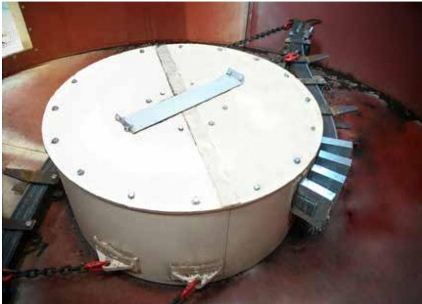
The machine is designed to remove the material at the bottom of a silo in order to favour dropping it into extraction screws.
