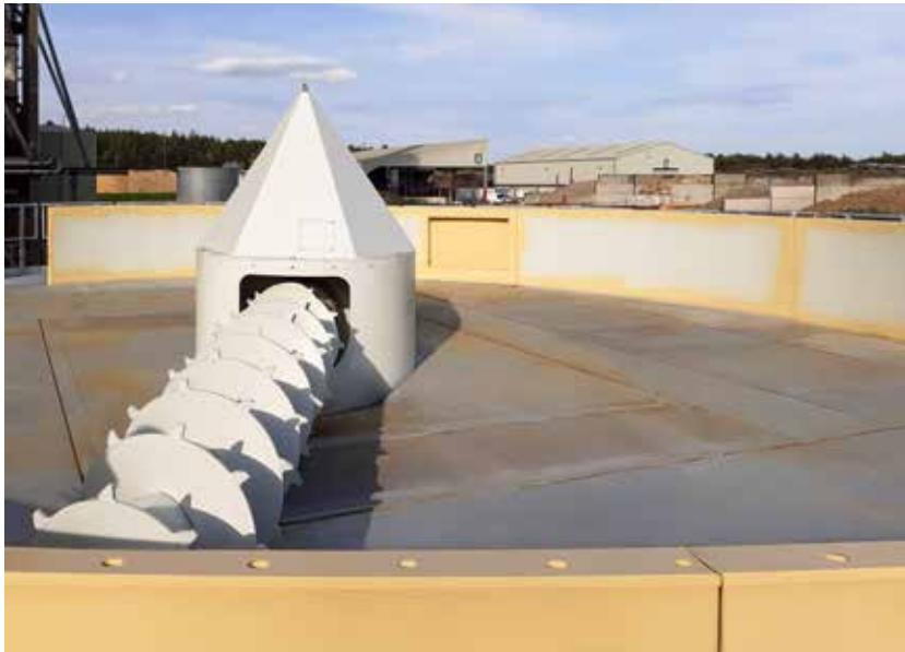
The machine is designed to extract wooden particles such as wood powder, sawdust, shavings and chips.
