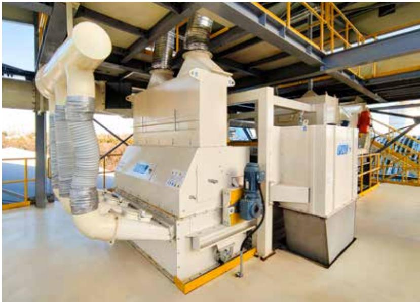
The machine is designed to separate non-ferrous electro-conductive metallic materials from inert materials, i.e. non-electro-conductive materials.
