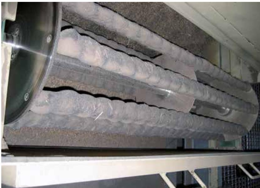
The machine is designed for continual and automatic separation of ferromagnetic materials, chips, particles, etc. and is connected directly to the output of the weighing unit of the main machine.
