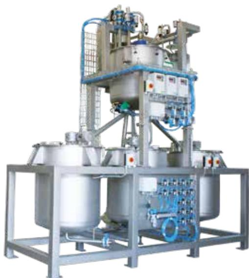
The WINGRAV9 gravimetric system designed for the preparation of resin mixtures for impregnation lines may be configured to suit a wide range of applications and requirements. The pre-programmed software may in fact be adapted to accommodate a large number of components, additives and utilities.
