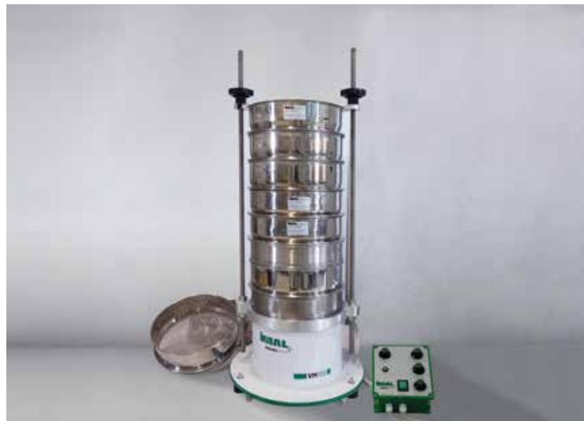
VM100 is an electro-magnetic impulse operated Sifter, controlled by a separate micro-processor with the following functions:
