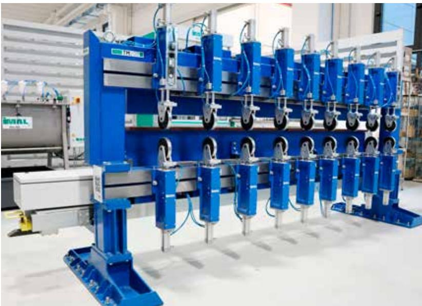
The TM200 system has been designed for the on-line measurement of thickness, weight and density (when used in conjunction with the weighing scale).
