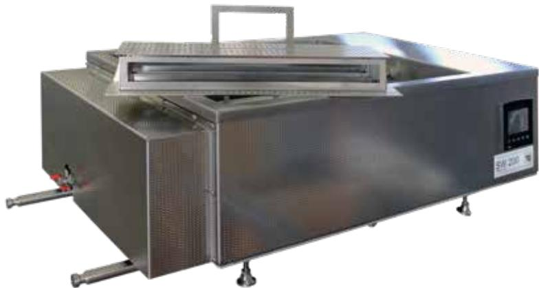
The SW200 and BT200 appliances consist of a water bath which is used to carry out laboratory and immersion tests on samples of wood-based panels (particleboard, MDF, OSB) in accordance with EN European standard requirements (it may also be used in conjunction with other IMAL equipment) such as: • Swelling and absorption (EN 317) • Boil test (EN 1087-1)
