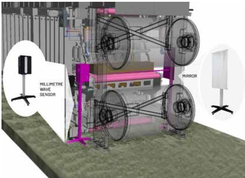
The SPF – Safe Press Feed system has been designed to control the mat at the infeed to the continuous press.
