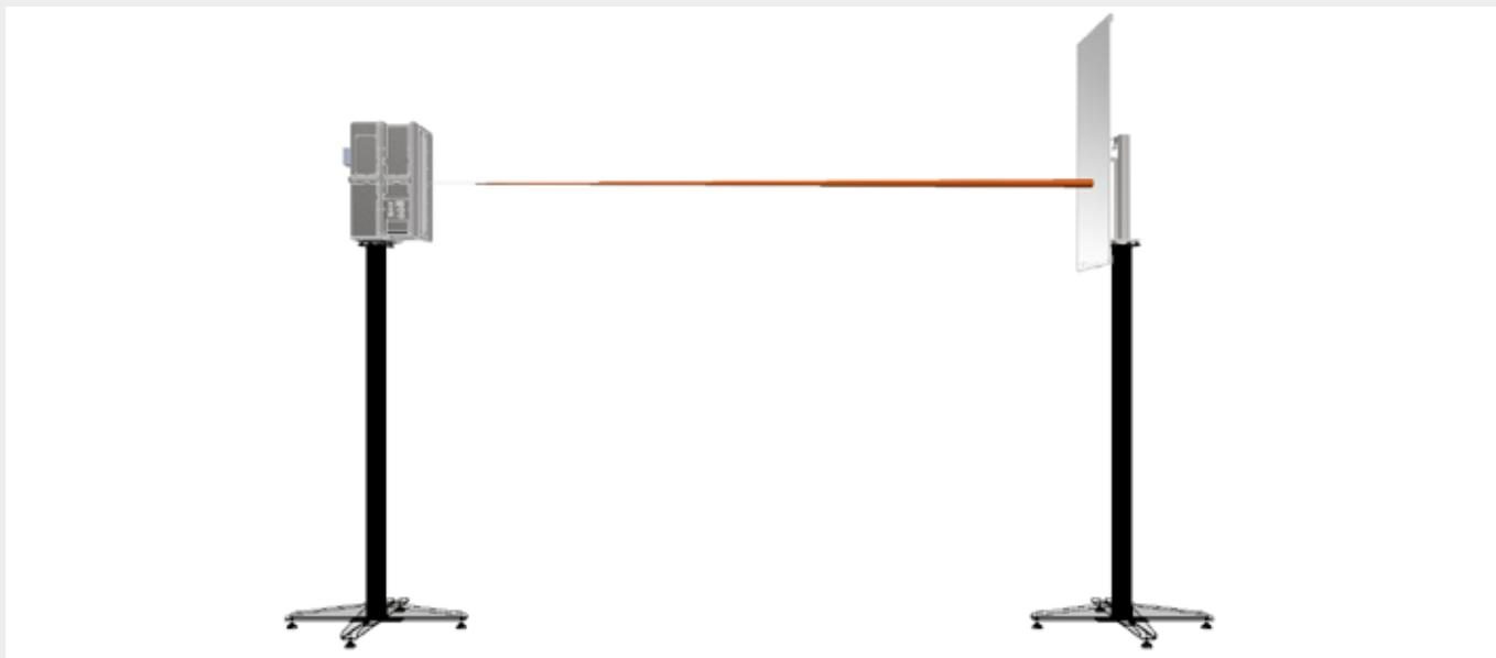
The SPF system works with millimetre waves and so it is completely safe for human health and can be operated without the need for any special permit from Health and Safety authorities or similar, unlike systems involving the use of X-rays
