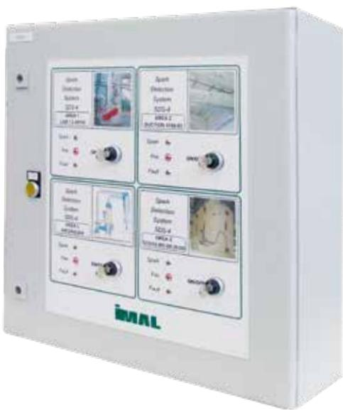
The SDS series spark detection and extinguishing system has been designed and developed to achieve spark detection in real time in all those environments where there is risk of fire (conveyors, filters, silos, screens etc.). The system consists of an I/O module that receives signals from the sensors and controls the opening of the extinguishing valves.
