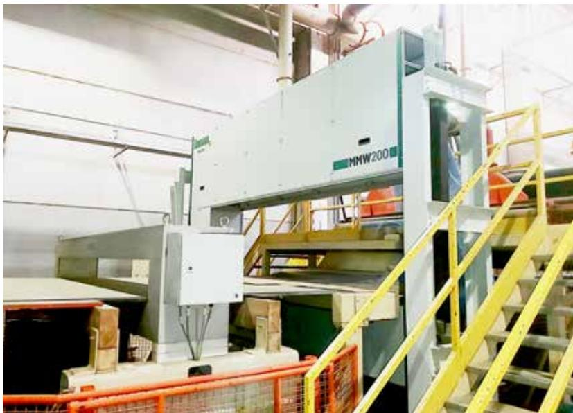
The system performs a rapid and continuous measurement of the weight per area, moisture content and thickness along the transversal section of the mat. It is normally installed just after the pre-press to monitor the formed mat. The analysis takes place without any contact with the mat and is perfectly safe for operators to use, thanks to the Terahertz technology, the same technology applied in the airport body scanner systems.
