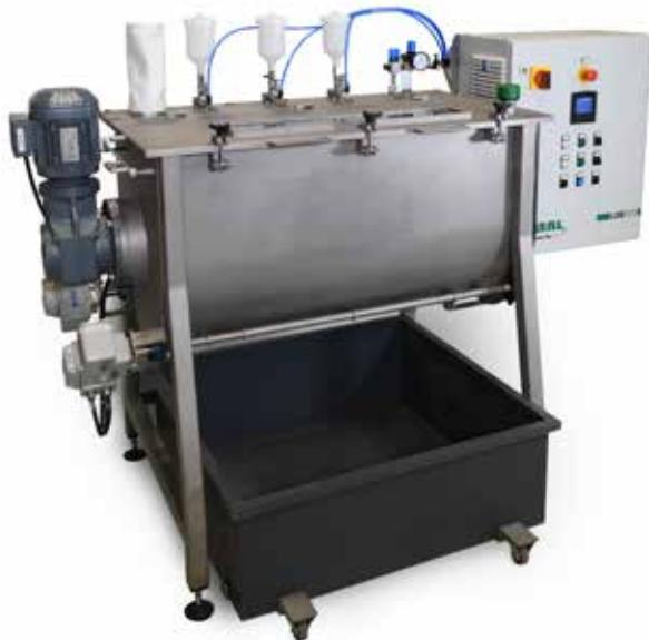
The glue blender, installed on a metal supporting structure, consists of a suitable sized drum, a top door for manually loading the material, and a bottom door through which the material is discharged. The mixing tools inside the drum are mounted on a shaft which is operated by a gear motor. Pneumatic nozzles spray the glue mixture onto the material.
