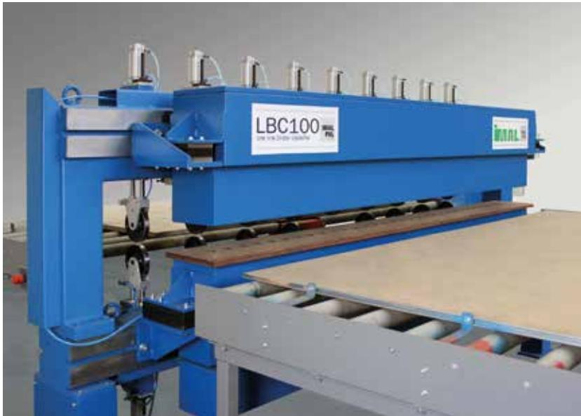
The LBC100 has been designed to detect unglued, delaminated, blown or low density areas, bubbles, cracks and other flaws inside any type of board (PB, MDF, OSB and Plywood).
