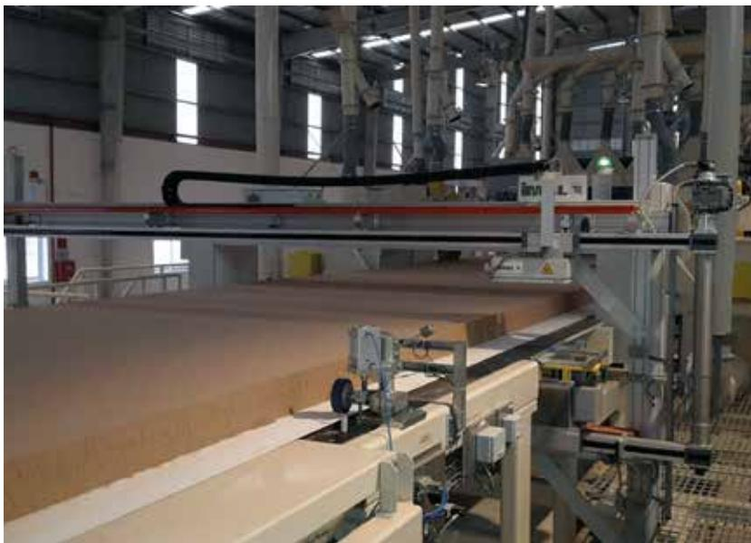
The system performs an accurate on-line surface density analysis (weight per surface unit) along the cross section of the mat being examined. It is also possible to measure lengthways, selecting a point on the mat where the scanner can be positioned automatically.
