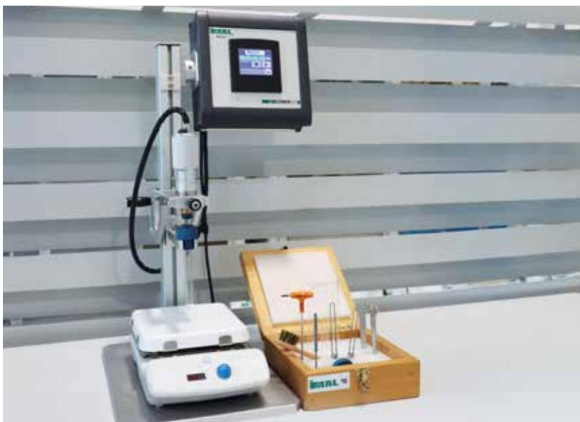
The Geltimer has been designed to measure the gel time of the resin delivered by the supplier and the gel time of the glue mix applied in the blender and the blow line.
