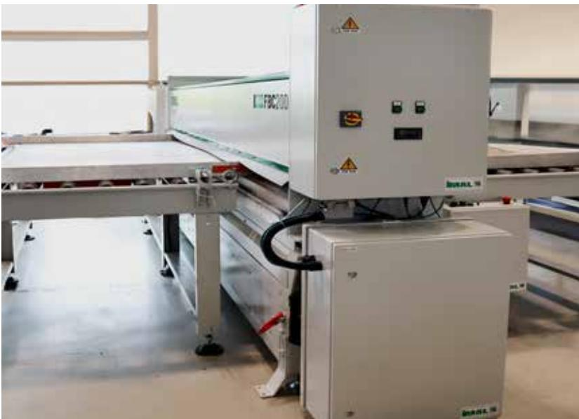
The FBC200 has been designed to detect unglued, delaminated, blown or low density areas, bubbles, cracks and other flaws inside any type of board (PB, MDF, OSB or Plywood).
