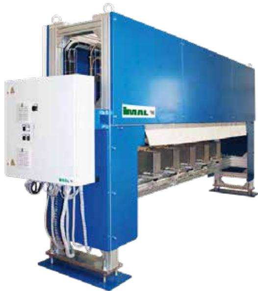
The system permits a continuous and reliable measurement of the weight per area ( $\text{kg}/\text{m}^2$ ) of the board, even at high speeds. The unit is equipped with "n" number of X-ray tubes, designed to ensure that the emission characteristics are suitable for these particular measuring requirements, combined with solid crystal receivers (the "state-of-the-art" in terms of X-ray receivers).
