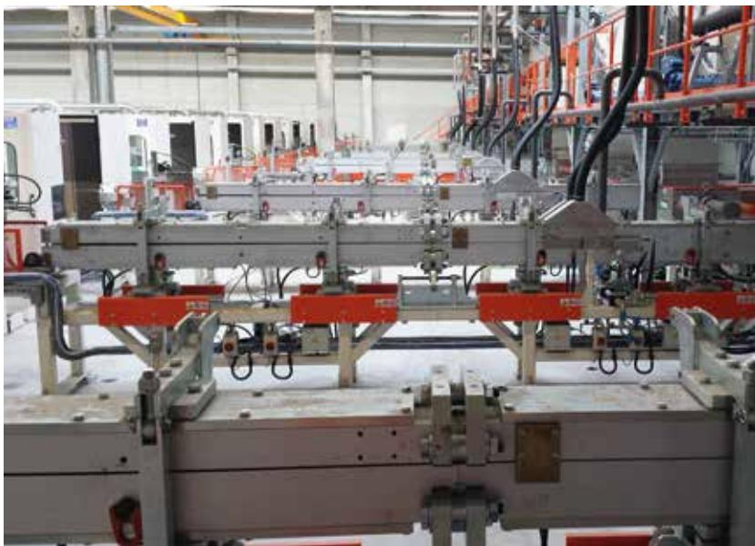
The extrusion press for pallet blocks production is able to produce all kinds of pallet blocks from all varieties of wood-based raw materials.
