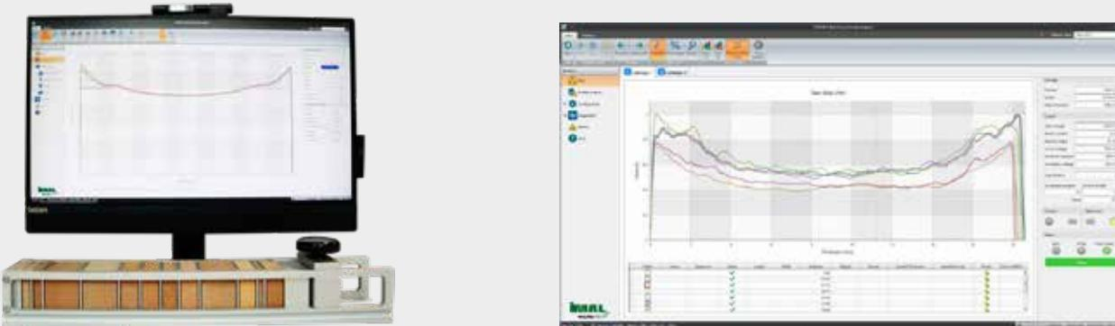
A smaller version is also available, the DPX400-LTE. The main difference to the standard version is that the dimensions in this case are measured by a digital calliper connected directly to the PC via USB and the sample holder is smaller, 200 mm, and not interchangeable. The two devices are identical in terms of X-ray analysis.
