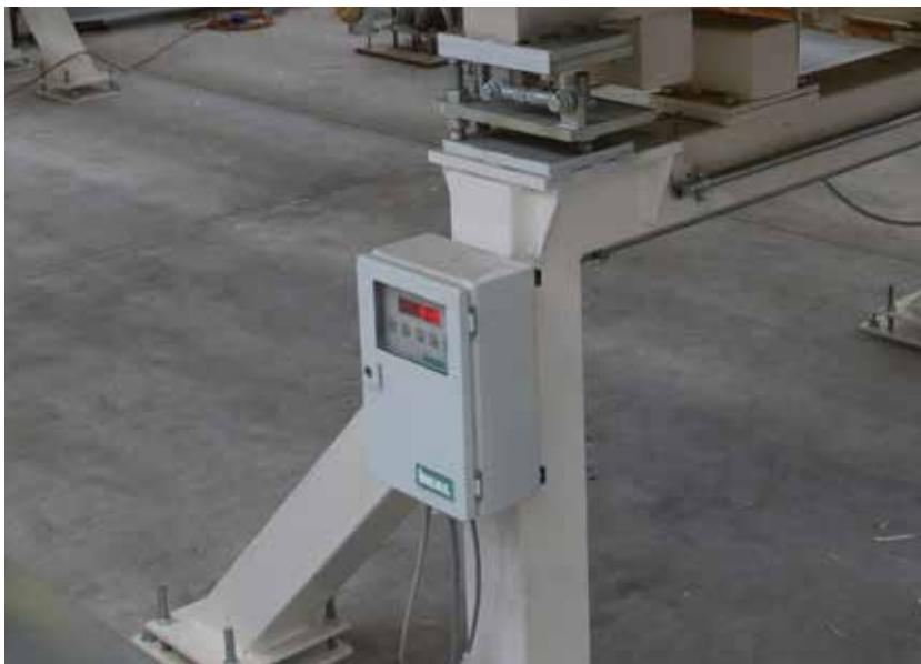
The BPP is a scale that has been designed for the continuous weighing of raw boards.
