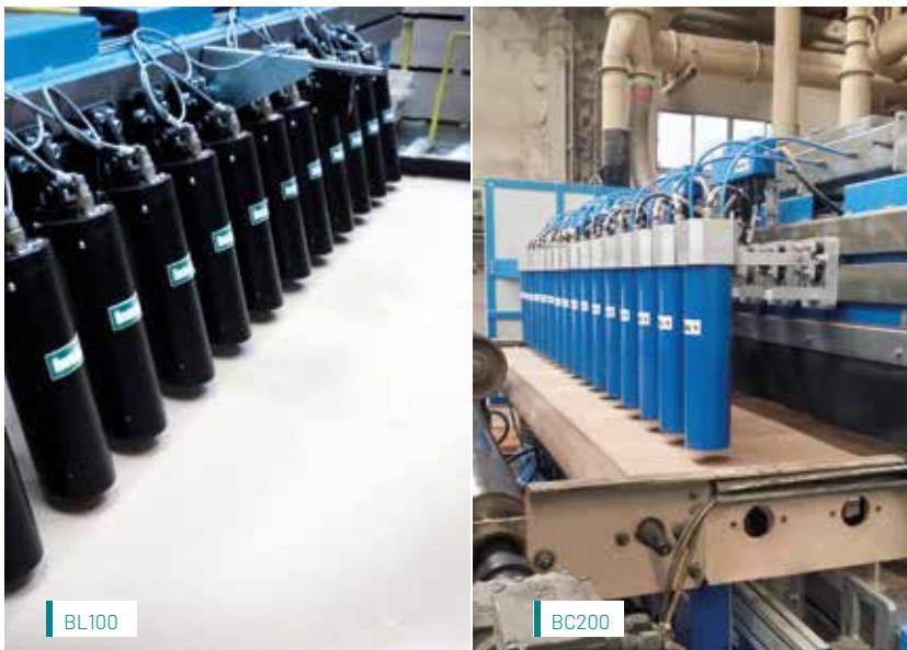
The IMAL BLISTER systems BL100 and BC200 have been designed for the on-line detection of flaws or imperfections which may occur in wood-based panels (particleboard, OSB, MDF, Plywood and LVL) such as unglued areas, blistered or blown areas, bubbles, cracks, etc.
