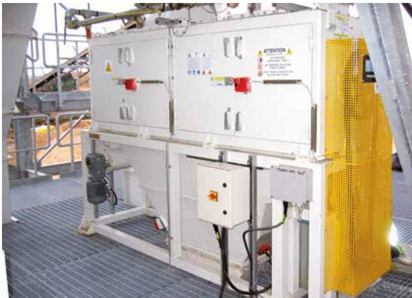
The machine is designed to select the incoming bulk material by its size. The first stage of the process is carried out in the Centrifugal Cleaner. The input material is separated from the finer particles, which are considered waste, by the centrifugal action of a rotor and filtration through fixed screens. The accepted wooden material, now free of any contaminants and within the required granulometric range, is collected in the output hopper.
