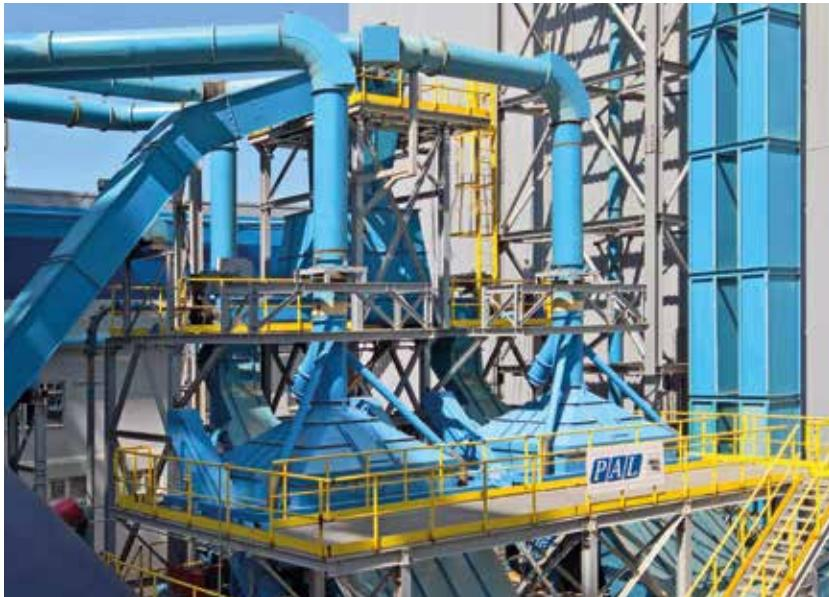
This machine is designed to separate heavy bodies, such as stones, glass or metal pieces, from the wood chips flow processed by the machine. This cleaning task is obtained by the combined action of vibration and air blowing.
