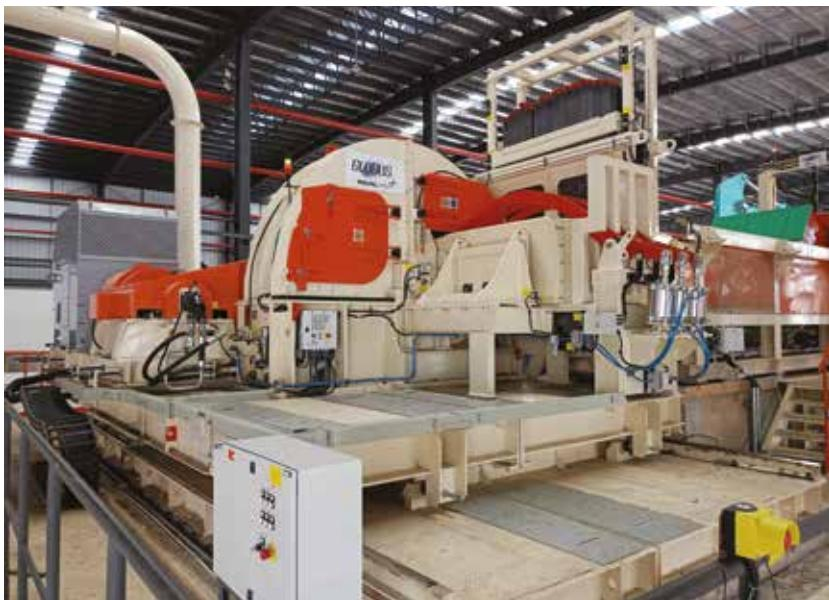
The machine is designed to process batch-fed logs into strands for OSB production.
