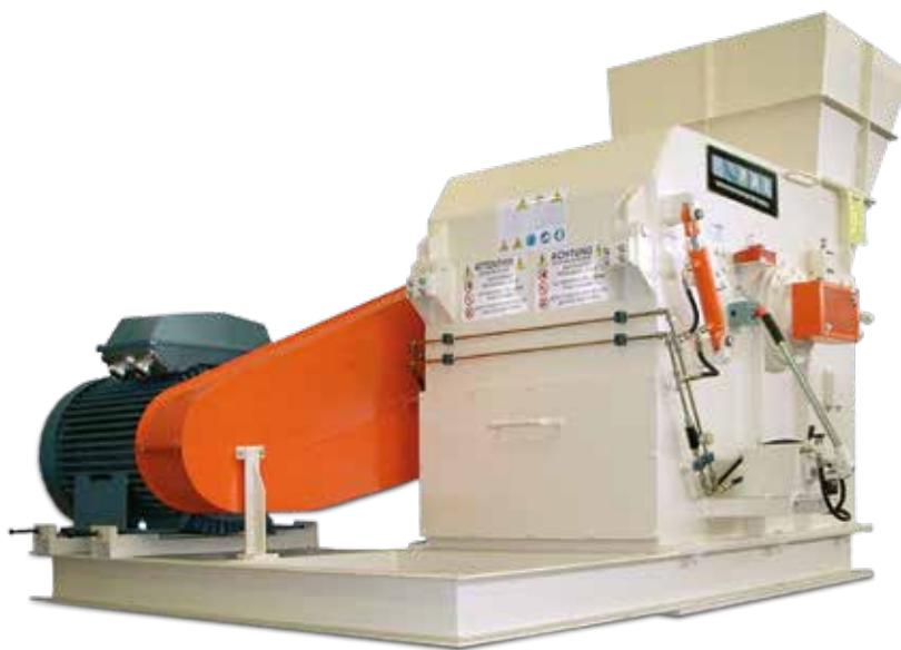
The machine is designed to reduce the chips of clean wood of various dimensions to uniform dimension chips.
