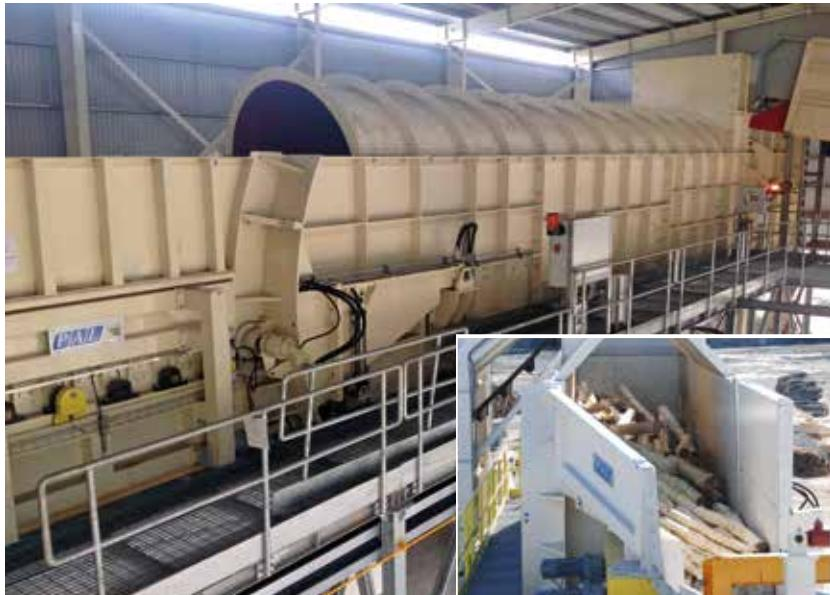
The machine is designed to remove the bark from trunks by the rotation of the rollers giving them at the same time a push towards the output where a toothed roller discharges the debarked trunk onto the next machine.
