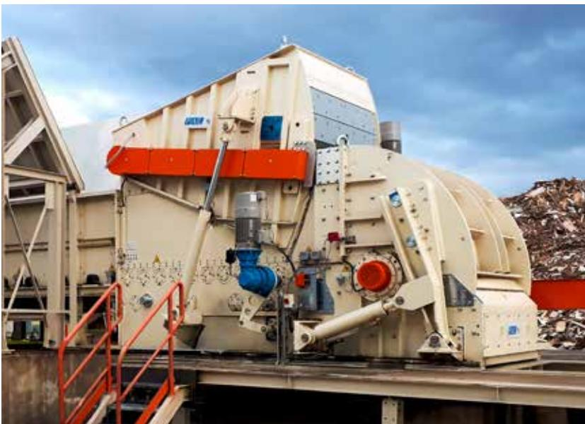
The machine is designed in order to break down recycled wood (off-cuts, pallets, scrap material) into different shapes and sizes in order to obtain finer material.
