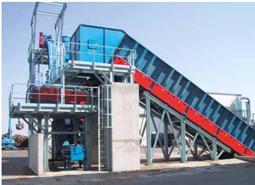
The machine is designed to convey wood trimmings of various sizes for processing.
